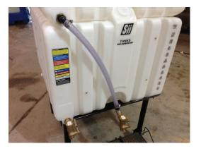
10. Fill each tank. Be sure to double check each fitting for leaks. Snyder is not responsible for fluid loss or clean-up costs.
