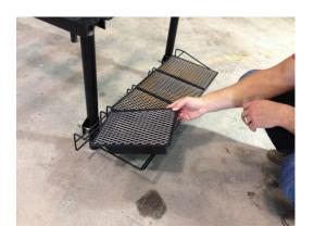
4. Attach elbow kit(s) to front lip of the stand base, using 1/2" wrench. Repeat as necessary.
