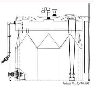
**Bolted and Threaded Manways** are available in sizes up to 24". Standard size is an 18" threaded manway.
