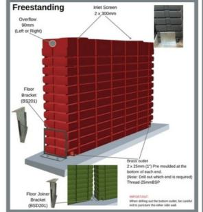
Multiple tanks connection fittings Fittings Brackets BS201 BSD201 Drill out Install the Install overflow install bucket 2 tanks connected with tank pipework and whichever end downpipe into the height tap(if to tank connection kit plumb away is required to inlet pre-fitted with required) put the ball from tank base leaf strainer. IMPORTANT valve or into storm Thread tape should be used on all couplings and ball valves. water
