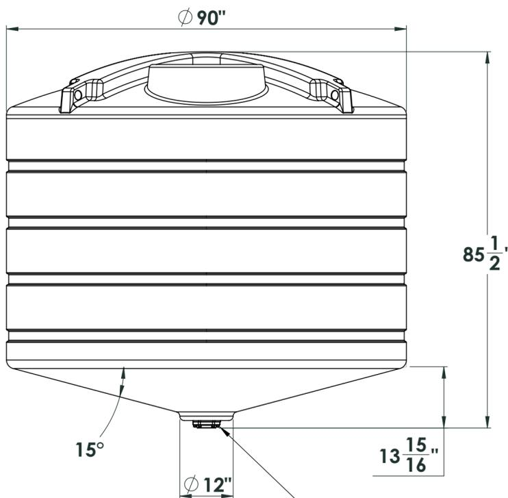
3 inch bolted - bottom drain fitting
