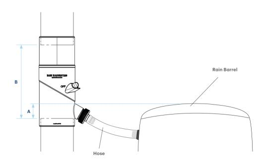
1. Select a position to install your downpipe diverter which will allow a smooth path for the hose to your barrel. If you are using the inlet hose to limit the height of water within your barrel, ensure the outlet is below the top of the rain barrel. Mark the lower cut point (A).
