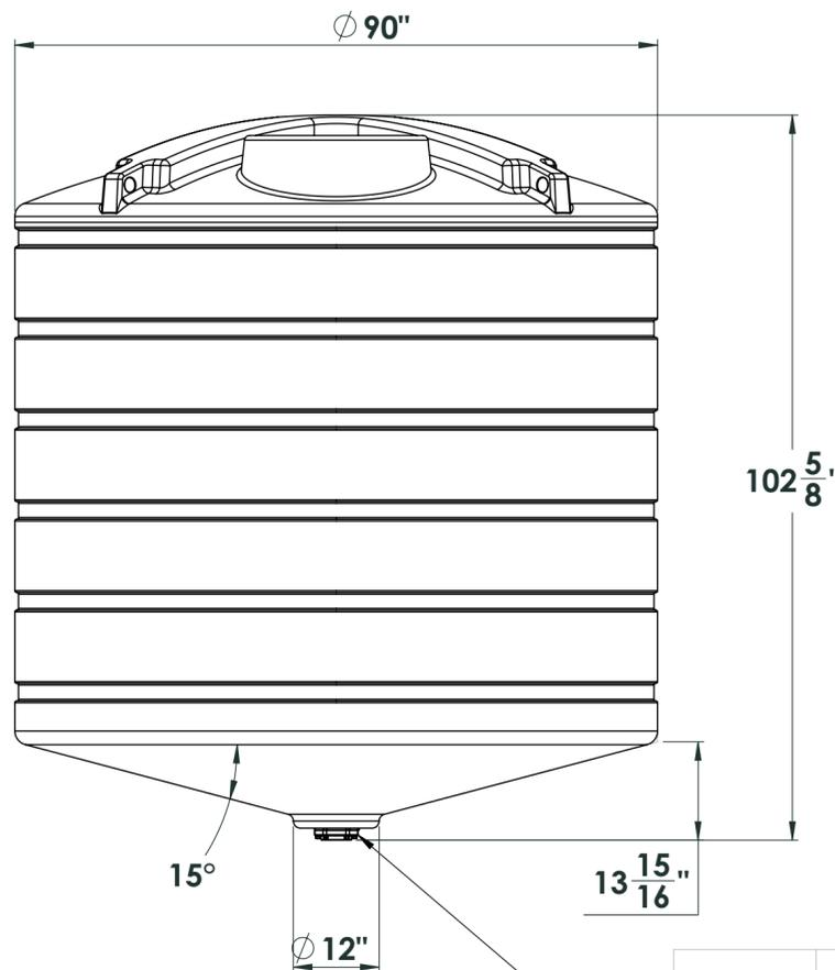
3 inch bolted - bottom drain fitting
