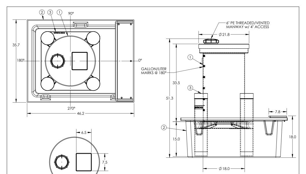
TANK SHOULD BE PLACED IN THE CENTER OF THE STAND WITH BLOCKS LOCATED BETWEEN THE TANK AND STAND COLUMNS FOR SUPPORT.
