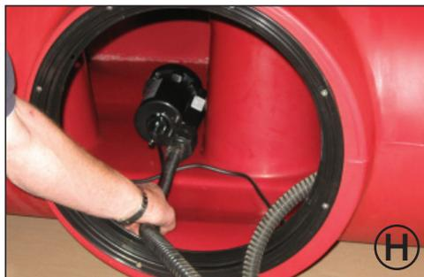
Place the pump back into the tank as shown. Ensure that the flexible hose is also inside of the tank.
