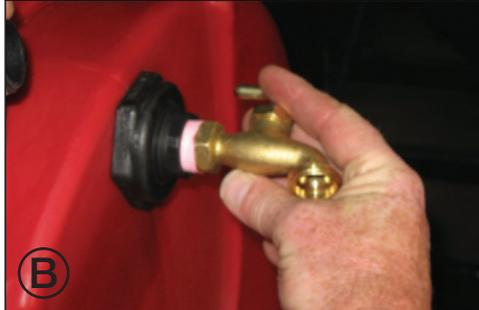
Attach the spigot to one of the ends and hand tighten. Using an adjustable wrench tighten the spigot another full rotation after hand tightening.
