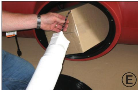
Carefully remove the downspout and lift the catcher box from the tank; set aside.
